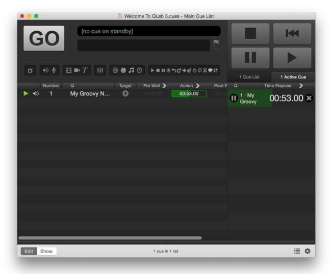
Each active cue is displayed in its own row, with its own controls. The row shows the cue number and name, and the elapsed or remaining time in larger text. You can toggle between showing elapsed time and remaining time by clicking on the chevron in the list header.
