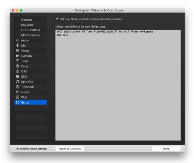
**Set new Script cues to run in a separate process.** Running scripts in a separate process improves QLab's performance while the script is running, but prevents QLab from tightly synchronizing with that script. For complex scripts or scripts that don't have an element of synchronization to them, we recommend keeping this box checked.
