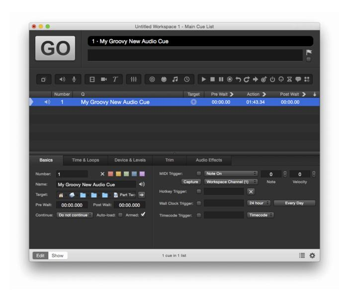
The settings on the left side of the Basics tab refer to basic properties of the cue. Many of the properties shown in the Basics tab are also editable from the Cue list.
