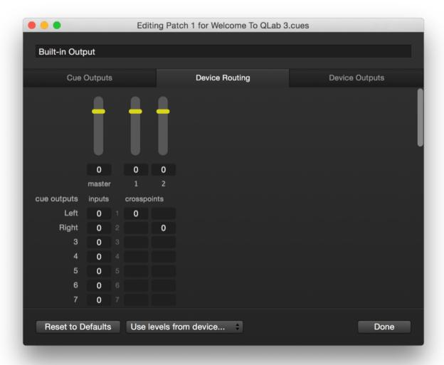
The Reset to Defaults button at the bottom restores the matrix to its default position.
