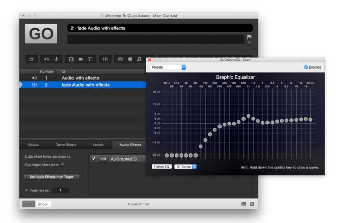
AudioUnits can also be placed on Cue Outputs and on Device Outputs, but effects there cannot be the target of Fade Cues. To learn more about effects on outputs, see <u>Settings</u>.
