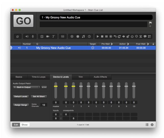
**Audio Output Patch.** Choose your output patch from the drop-down menu in the top-left corner of the *Device and Levels* tab. The … button directly to its right a shortcut to the Patch Editor for the selected patch. Generally, you won't need to touch this after you set it up for your show. You can <u>learn more about</u> the <u>Patch Editor</u> in its section of this documentation.
