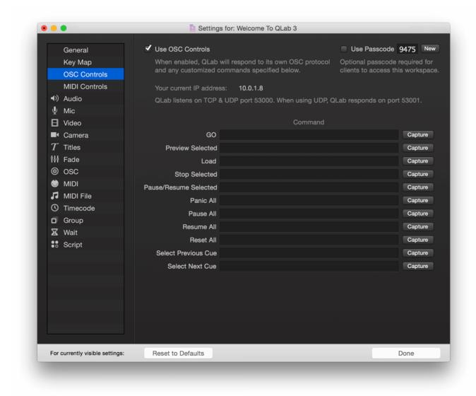
**Use OSC Controls.** When enabled, QLab will respond to its own OSC protocol as well as any customized commands for the transport controls listed below.
