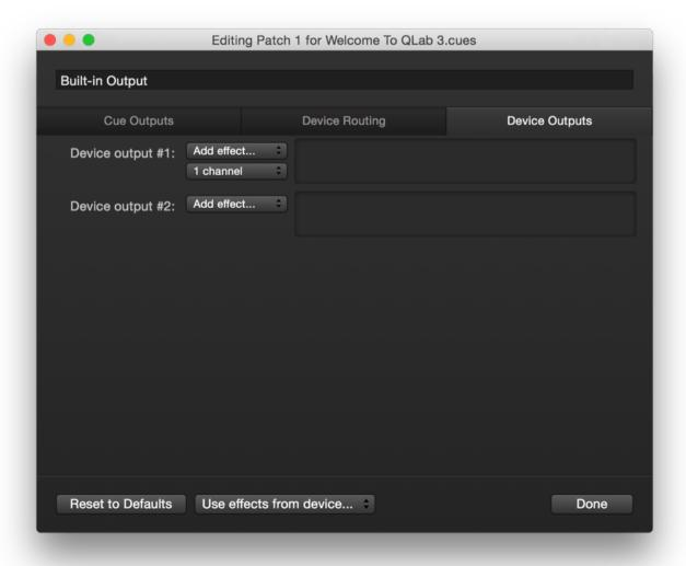
The *Use effects from device...* button shows a list of any audio devices that have ever been attached to this workspace, and selecting one attempts to duplicate the arrangement of AudioUnits used with that device when it was last connected.
