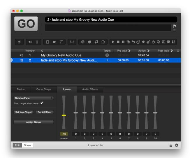
In this screen shot, the Fade cue reduces the master level of the target cue by 10 db. If you run the Fade cue twice, the master level of the target cue will end up -20 below its starting level.
