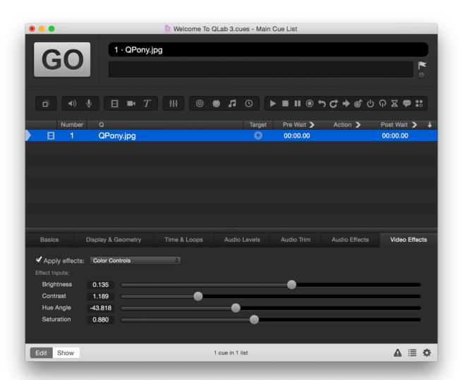
QLab comes with a variety of video effects pre-installed. You can also create your own effects using Quartz Composer. For a composition to be compatible with QLab, it must be an effect (which is one of several types of compositions that Quartz Composer can create) and it must publish an input named \_protocolInput\_Image which is where QLab will send video to the composition, and \_protocolOutput\_Image which is where QLab will receive the effected video from the composition.
