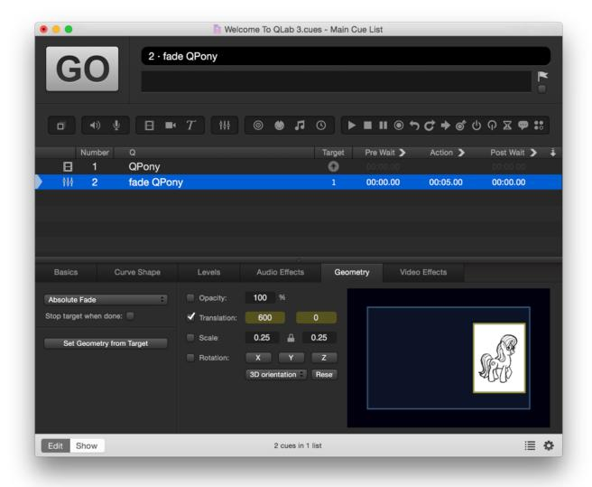
By default, the checkbox next to each parameter will be unchecked, meaning that the Fade cue will not adjust that parameter. To fade a parameter with the Fade cue, just check the box next to that parameter.
