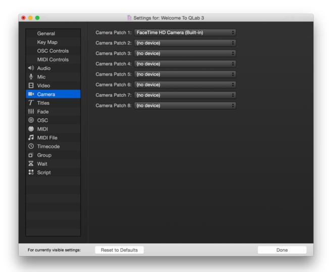
**Camera Patches.** QLab workspaces can connect to eight individual video input devices, which are assigned to one of eight Camera Patches. Use the drop-down menus to assign a device to a patch.
