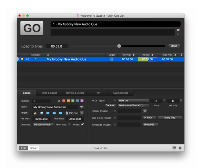
To use the Load to Time tool, type a number into the text field or drag the slider along the timeline to load the selected cue or cue sequence to your desired time.
