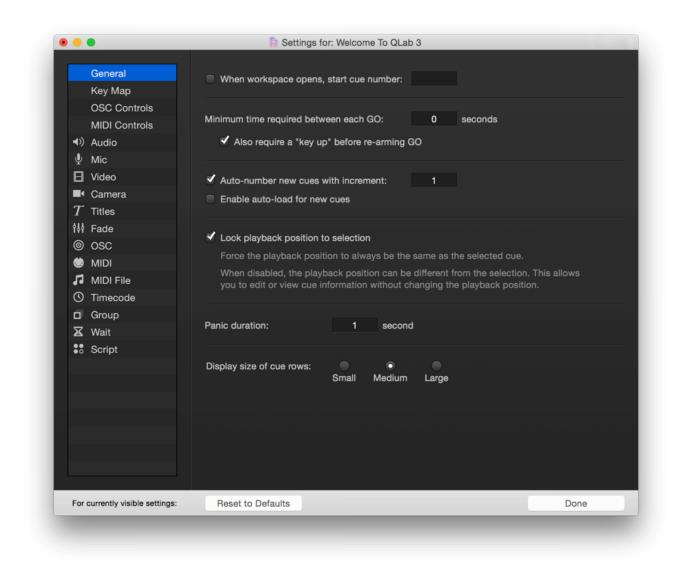
When workspace opens, start cue number. Check this box and enter a cue number in the text field, and QLab will automatically start that cue when this
