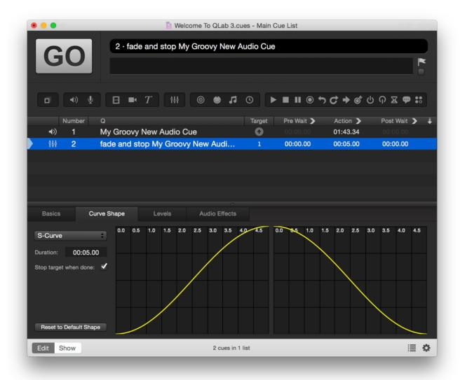
Check or uncheck the *Stop target when done* box under the Duration text field depending on whether you would like the target cue to continue playing after the Fade cue is complete, or stop once the Fade is complete.
