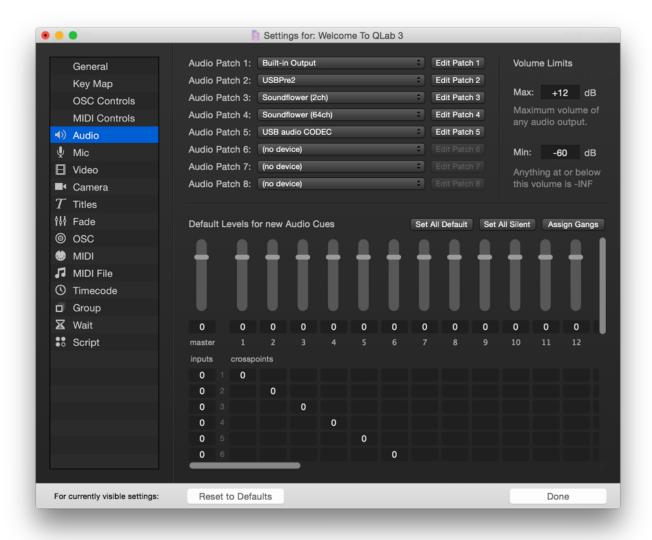
**Audio Patches.** QLab workspaces can connect to eight individual audio devices, which are assigned to one of eight audio patches. Use the drop-down menus to assign a new device to a patch. Click the *Edit Patch* buttons to the right of each drop-down menu to edit the details of that audio patch.
