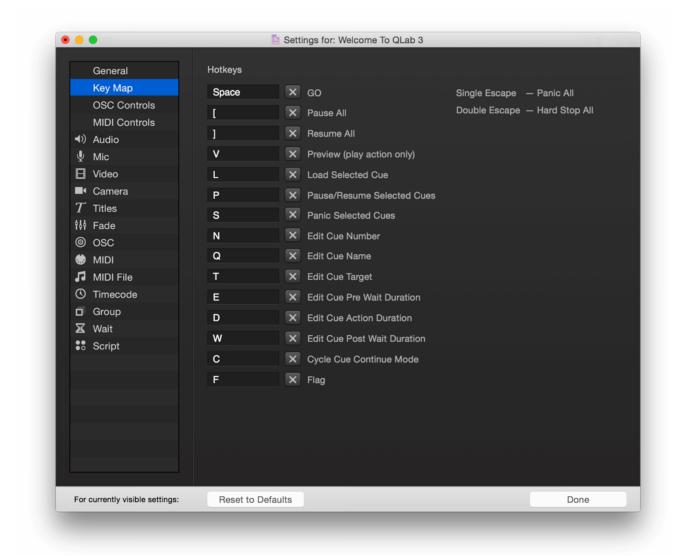
The Key Map allows you customize keyboard shortcuts, or hotkeys, for the listed commands. Simply enter the desired hotkey in the text field next to the appropriate command. To disable a hotkey, press the X button next to the command.
